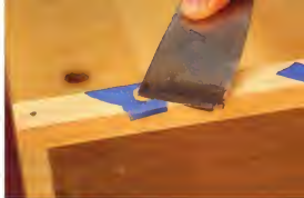
Shot through the tape. Masking tape ensures any wood filler is directed into the hole only and not into the surrounding wood pores.
